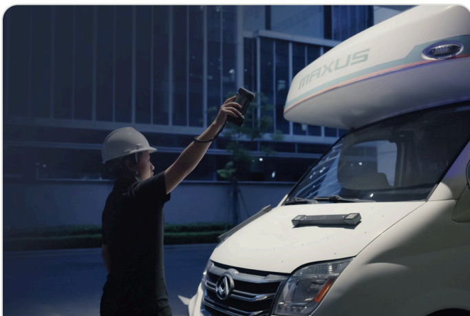
Built-in VPG on a camper van. Scale bars on the hood set the reference while the scanner builds the frame.
