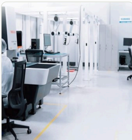
Calibration benches: instruments are verified to VDI/VDE 2634 and ISO 10360 before a certificate is issued.
