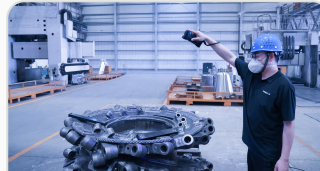
Heavy industry: a large casting scanned where it sits.
