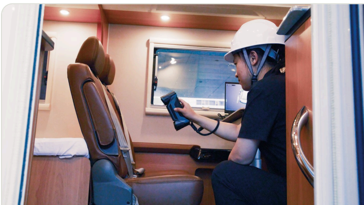
IR rapid scan inside a camper van. Seats and cabinetry are captured quickly with no markers.
