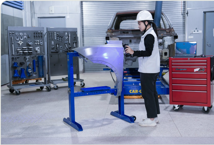
A car fender scanned in its fixture. The data goes straight into SHINING3D Inspect for a color map and report.
